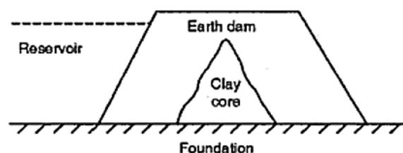
Embankment dams come in two types: the earth-filled dam (also called an earthen dam or terrain dam) made of compacted earth, and the rock-filled dam. A cross-section of an embankment dam shows a shape like a bank, or hill. Most have a central section or core
