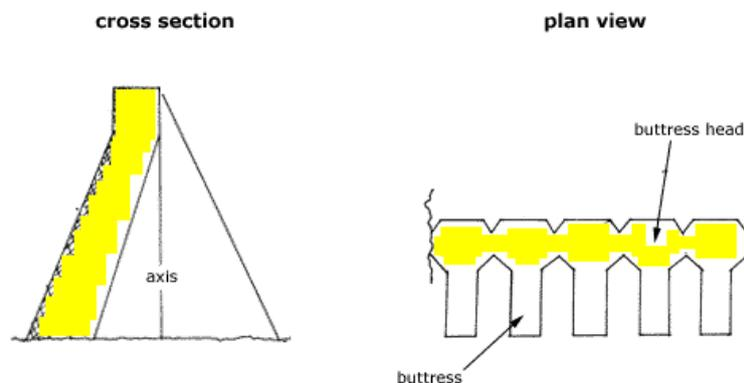
Buttress or hollow gravity dams were originally built to retain water for irrigation or mining in areas of scarce or expensive resources but cheap labour. A buttress dam is a good choice in wide valleys where solid rock is rare.
